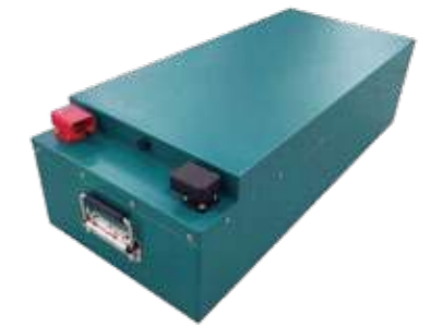
Model: FEB72110(24S) Parameter: 72V 110Ah Dimension: 700x306x200mm Weight: 64±1kg
